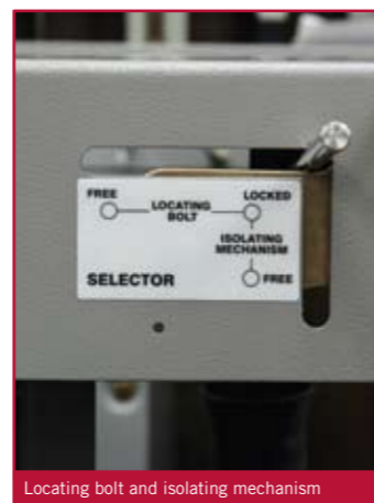
Locating bolt and isolating mechanism
